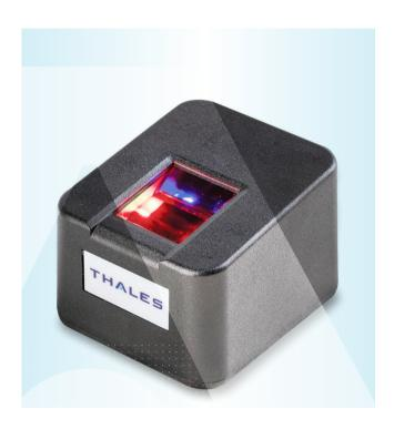
The Cogent Single Finger Scanner DactyID20 is a compact single-finger livescan offering a superior built-in fake fingers detection system. This makes the Cogent Single Finger Scanner DactyID20 the best choice especially for unattended applications like kiosks, pc/network-login, time and attendance and many others.
