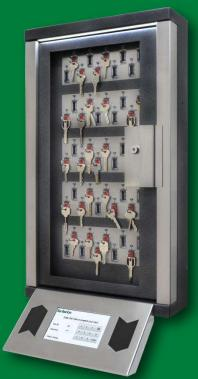
The keys are attached to intelligent keyfobs that have a built-in chip with a unique identifier and a three-millimeter stainless steel shackle. The data from the built-in chip is used to verify and identify the key every time you need to remove the key from the storage or put it back to its place. Only authorized users, whose rights are assigned individually, can have the access to a key. Keyfobs of different colors are available for order.
