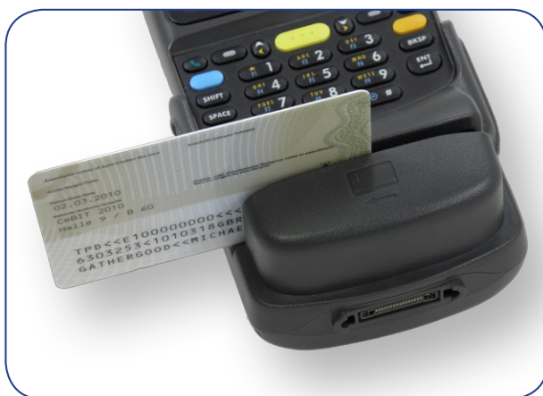
The OCR310-MC7m reading an ID card
