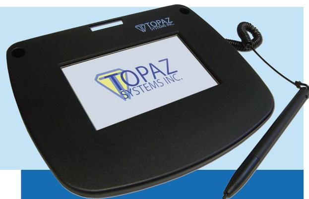
The Topaz SigLite® Color 4.3 is an advanced electronic signature pad with 4.3 inch, full-color TFT VGA (480 x 272) LCD that captures and displays “electronic ink” under the pen tip for a natural signature. Bundled secure software APIs provide for interactive text, graphics, and pen-tap hotspots and checkboxes which enable users to navigate screens, read agreements, and select preferred options before signing.
